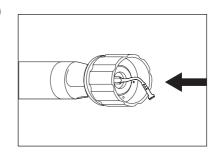
Place the insert into the wrench as shown;
