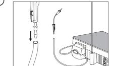
Connect the flow adjuster (not supplied) to the liquid bag used for the treatment (bag not supplied). Hang the bag to its specific support rod;
