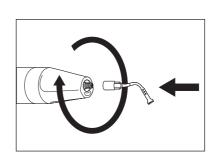
Tighten the insert by using the PIEZOSURGERY/Mectron torque wrench. To correctly use the PIEZOSURGERY/Mectron torque wrench, operate as follows:
