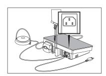
Equipotential plug: The device is equipped with an additional equipotential plug located on the rear of the console.
