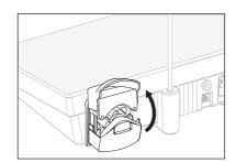
Insert the part of the irrigation tube with a bigger diameter and with length of 15 cm into the peristaltic pump;
