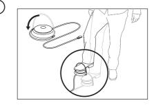
Connect the foot pedal to the back of the device in the socket marked with the symbol ≱, by means of the plug of the pedal cable, until you hear a "click" sound.
