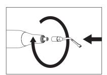
Use the Mectron torque wrench to secure the insert;
