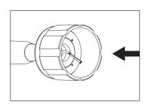
Fit the insert into the wrench as shown;
